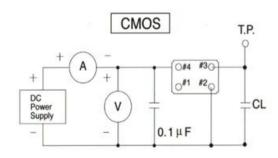
\*\*\* Because S21 series has no by pass capacitor. So, we recommend our customer to use capacitor 0.1µF in join Vcc and GND.
