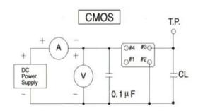
\*\*\* Because S21 series has no by pass capacitor. So, we recommend our customer to use capacitor 0.1µF in join Vcc and GND.
