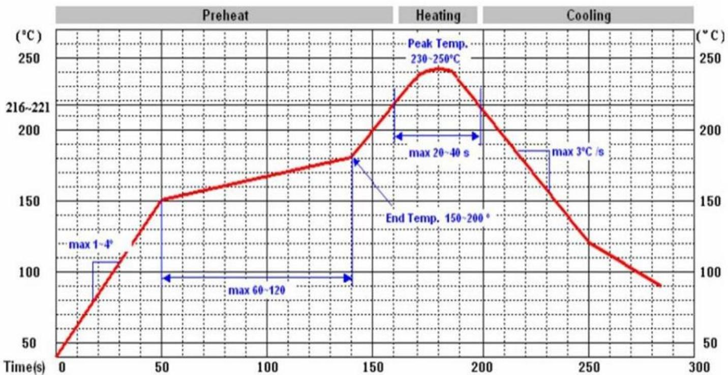
★ The absolute maximum reflow temperature is 260°C. Repeated reflow soldering processes or soldering the module upside down are not recommended.
