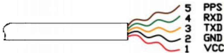
Figure2-1: Pin Assignment
