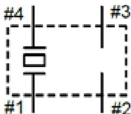
Pin #2 and #3 to be OPEN electrically to the PCB.
