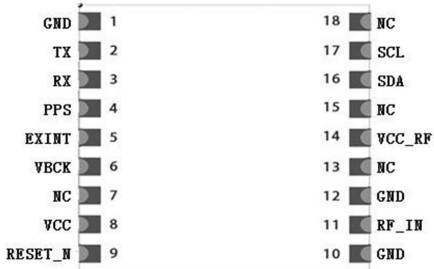
Figure 2: Pin Assignment
